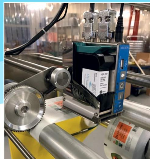
The HSAJET® Print & Verification solution is available as an integration kit as well as turnkey systems for both un-folded and folded cartons, blister packs and labels.
